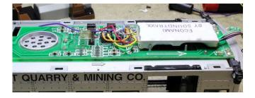
I wired the decoder directly to the 8 pin socket as shown. If you ever need to remove the decoder, use the plug at the decoder end of the harness.
