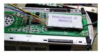
I used double side tape (the Black kind) to hold the decoder in place as shown. I fits nicely in place. This is the ECO 200 – UK but the ECO 100 – UK is smaller and fits well.
